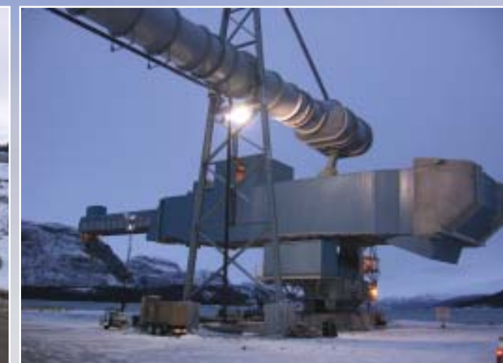
ABOVE LEFT: The 8mil (.0088", 200 micron) thick Barrier Series coating resists attack by alkalis, acids, salts and bleaching agents. The textured coating also resists coating impact damage. ABOVE RIGHT: Ship loader for Nickel, Copper and Cobalt ore.
